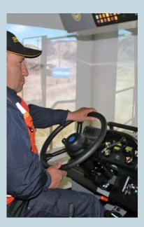
**Simulator cabins:** For operator training, preparing them to respond correctly to the main risks when driving mining equipment.
