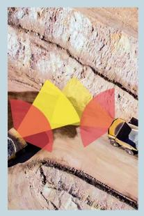
**Collision avoidance system (CAS GPS):** A system that detects near-by vehicles and mobile equipment, warning the driver on a screen with progressive audible and visual warnings.
