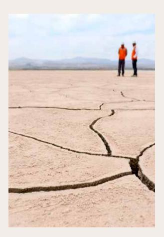
Any process to separate minerals from rock produces significant amounts of waste material that must be safely deposited in mining dumps or dams. At Michilla, Antucoya, Centinela Cathodes and Zaldívar, this is spent ore. At Los Pelambres and Centinela Concentrates it is tailings.
