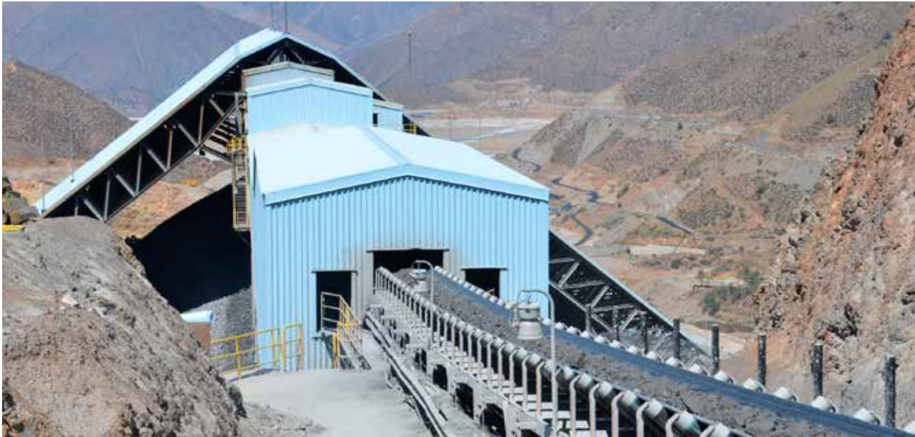
Since 2000, Minera Los Pelambres has used the energy generated by braking the conveyor belts (carrying ore from the mine to the plant) to generate electricity.
